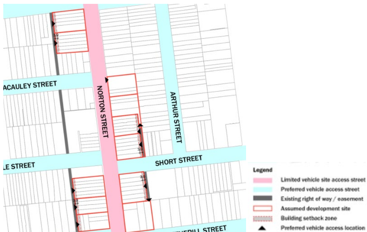
Figure 4.13.2 Norton Street North Precinct Preferred Access Arrangements
