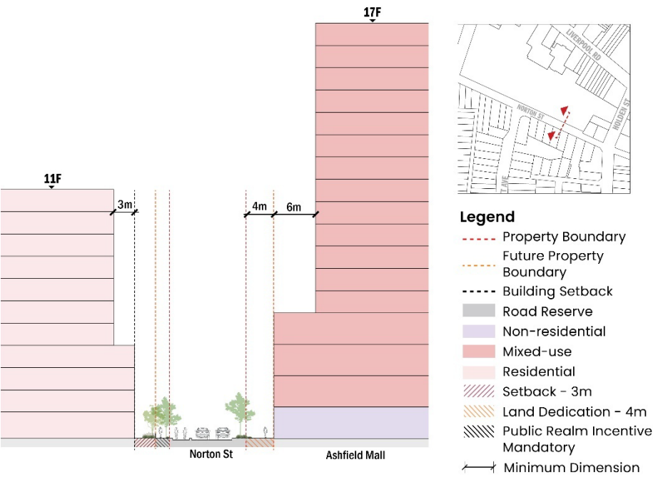
Figure 4.2.33 Ashfield Town Centre – Norton Street Section (17 Storeys)
