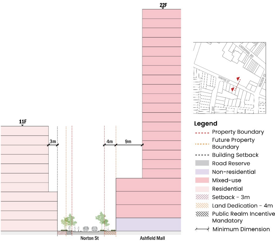
Figure 4.2.34 Ashfield Town Centre – Norton Street Section (22 Storeys)
